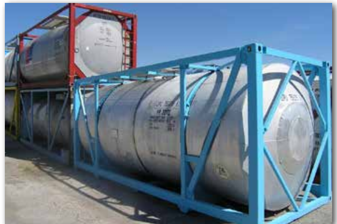
Heresite lining protects iso-tanks from harsh chemicals.
